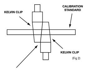
**NOTE:** Make sure clips are as close together as possible. Use the tips of the Kelvin clips when performing measurements on small diameter wire.
