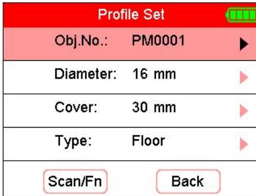
Figure 3.13 Profile scan setting interface
