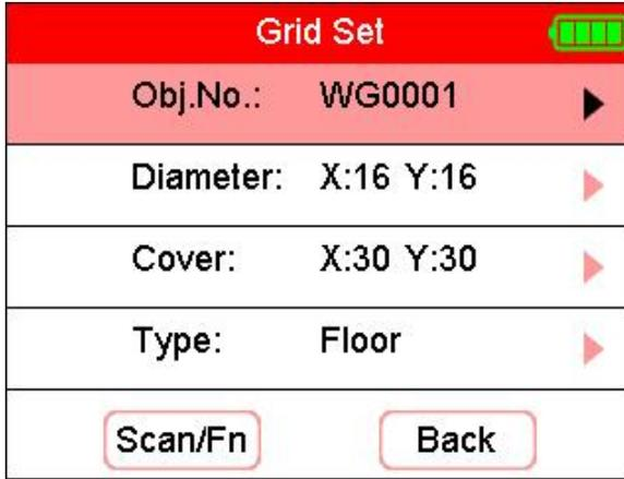
Figure 3.11 Grid scan setting interface
