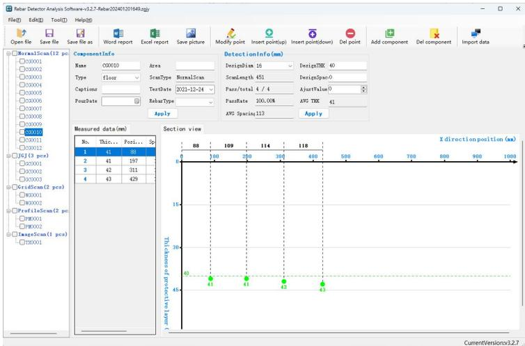
Figure 5.5 Rebar Detector analysis software interface
