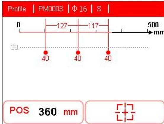
Figure 3.14 Profile scanning detection interface
