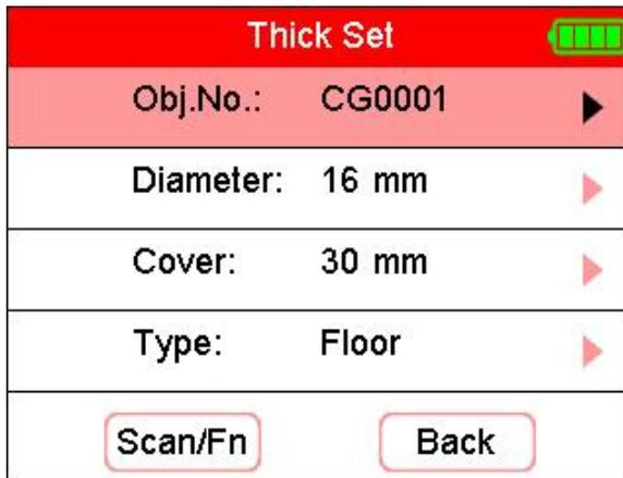
Figure 4.4 Thickness detection setting interface
