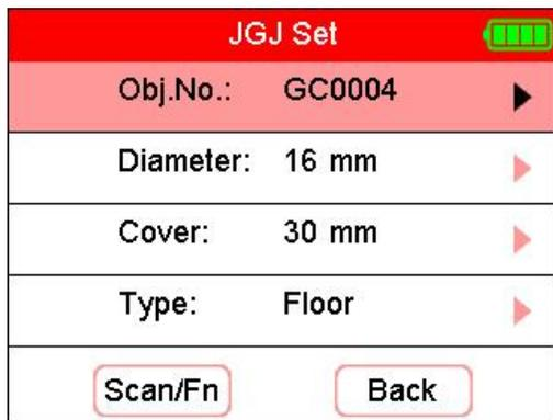
Figure 3.9 Procedure detection setting interface
