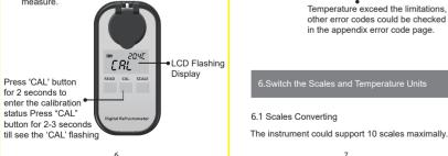
Press "CAL" button once again during the 'CAL' flashing to start to calibrate. When the calibration is completed showing as following. If no any operations for 10seconds the instrument would return back to booting status.
