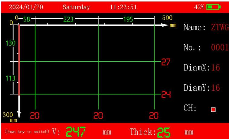
**Figure 3.9 Grid scanning interface**
