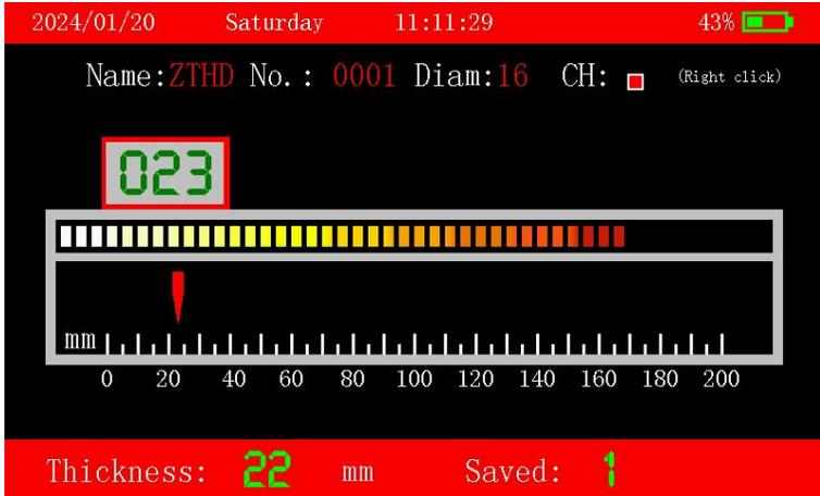
**Figure 3.6 Single point test - thickness test**
