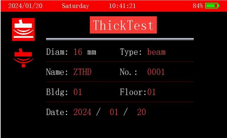
**Figure 3.3 Thickness Test Setting Interface**
