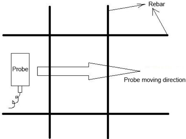
**Figure 3.5 Schematic diagram of probe movement**
