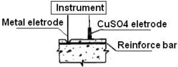
Diagram 2-8 Potential Test of the Steel Corrosion Meter
