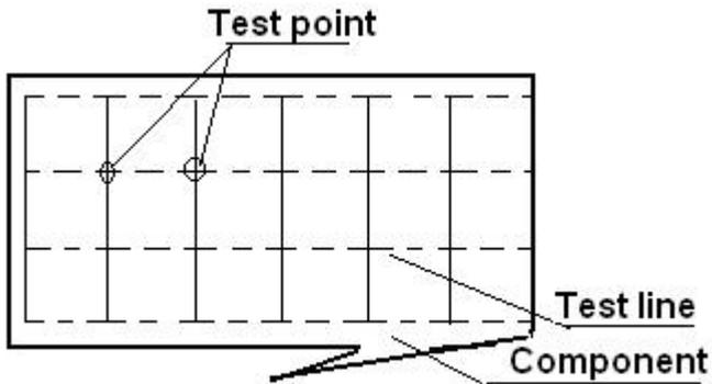
Diagram 2-7 Arrangement of Test Area and Test Point
