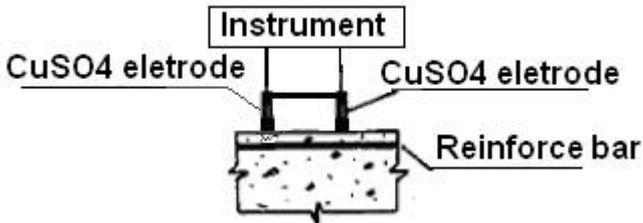
Diagram 2-9 Gradient Test of the Steel Corrosion Meter
