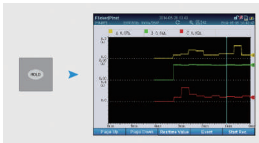
Figure 10-3. Cursor appearing when the Trends screen being in hold state
