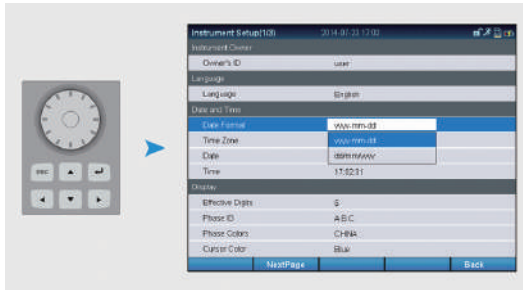
Figure 2-3. An instrument setup item with a selectable option
