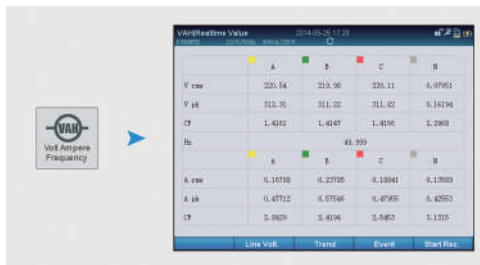
Figure 4-1. Realtime Numerical Values screen in the VAH mode
