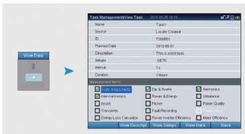
Figure 16-11. Viewing the Contents of a Task – View Data
