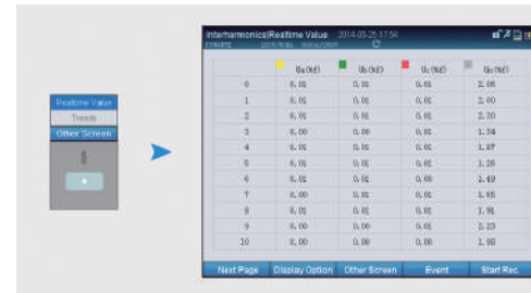
Figure 7-3. Realtime Numerical Values screen in the Interharmonics mode
