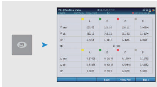
Figure 4-7. A sample screen after “” shortcut key being pressed
