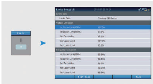
Figure 2-8. Limits Setup screen
