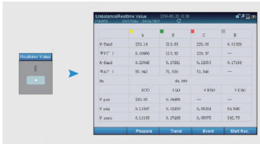
Figure 9-2. Realtime Numerical Values screen in the Unbalance mode
