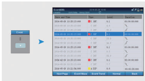
Figure 9-5. Events screen in the Unbalance mode
