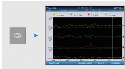
Figure 14-2. Cursor appearing when the Trends screen being in hold state
