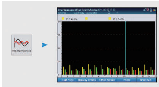
Figure 7-1. Bar Graph screen in the Interharmonics mode
