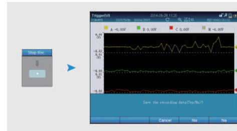
Figure 14-6. Stop recording data to a file in the Trigger Parameter View mode
