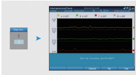
Figure 7-10. Stop recording data to a file in the Interharmonics mode
