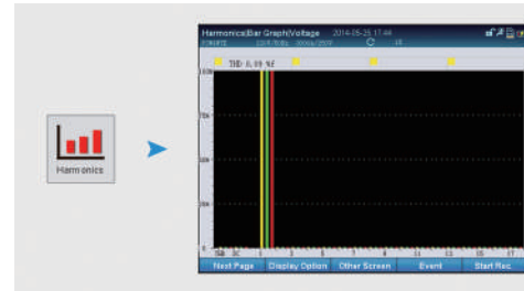
Figure 6-1. Bar Graph screen in the Harmonics mode
